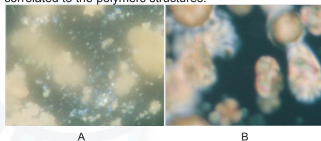
Figure 63 Photomicrographs of polymer 86b in heating cycle at (A) <109°C, (B) >112°C. 57
