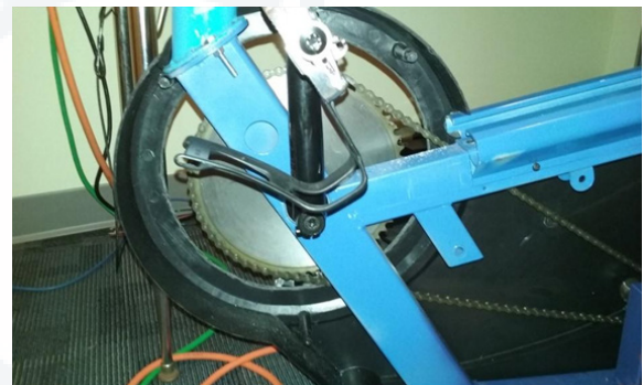
Figure 2: An industrial strength chain connected the gear reducer to the motor unit assembly. The crank spindle was 22mm in diameter, the pedals were platform, and the sprocket was bolt-driven with 58 1/8" teeth.
