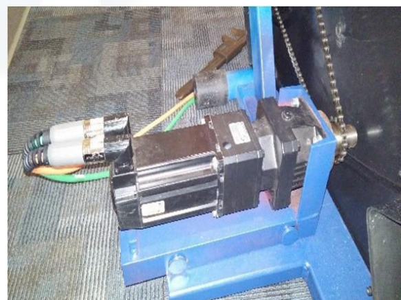
Figure 3: The ServoPro motor unit is attached to the cycle with the assembled mounting bracket.
