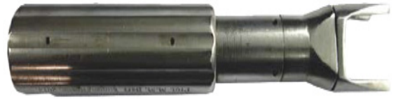
Figure 4.32 : Direct Measuring wire tensioner (Russian Dynamometer)
