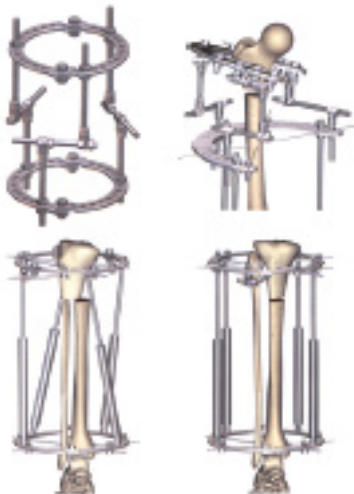
Diagrams of the Ilizarov fixator configuration to correct rotational deformities
