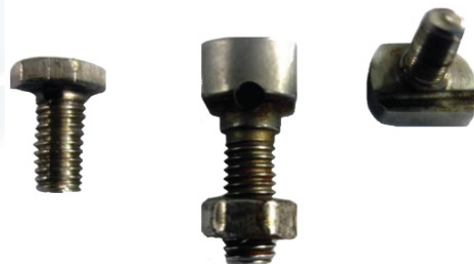
Figure 4.21 : Nuts in slotted and cannulated bolts.
