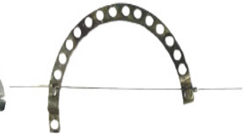
Figure 4.39 : Use of buckles to fix additional wires.
