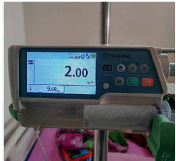
Figure 20.8 Syringe pump is used for accurate dose calculation in inflow tract of CLAP therapy.
