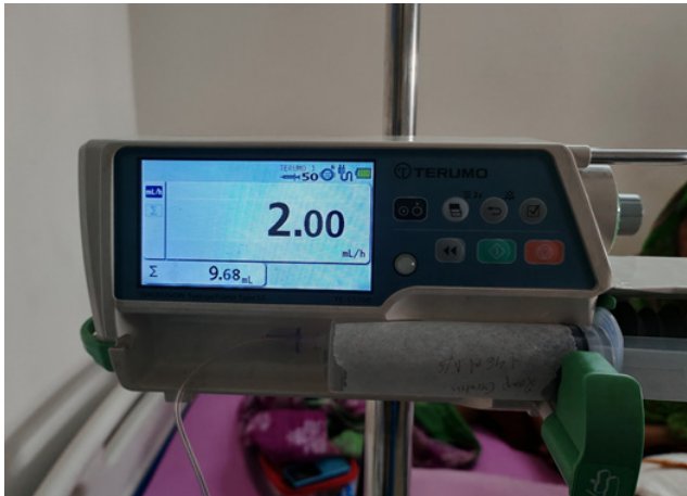
Figure 8 Syringe pump is used for accurate dose calculation in inflow tract of CLAP therapy.
