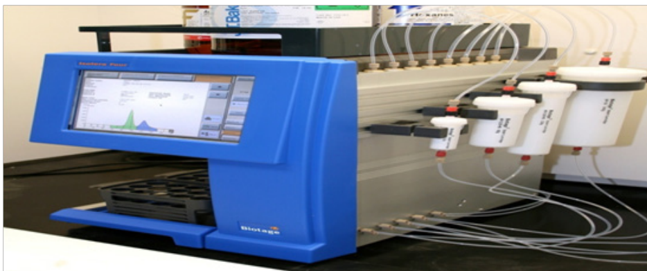
Figure 5: Biotage (Isolera one), Flash Chromatography System.
