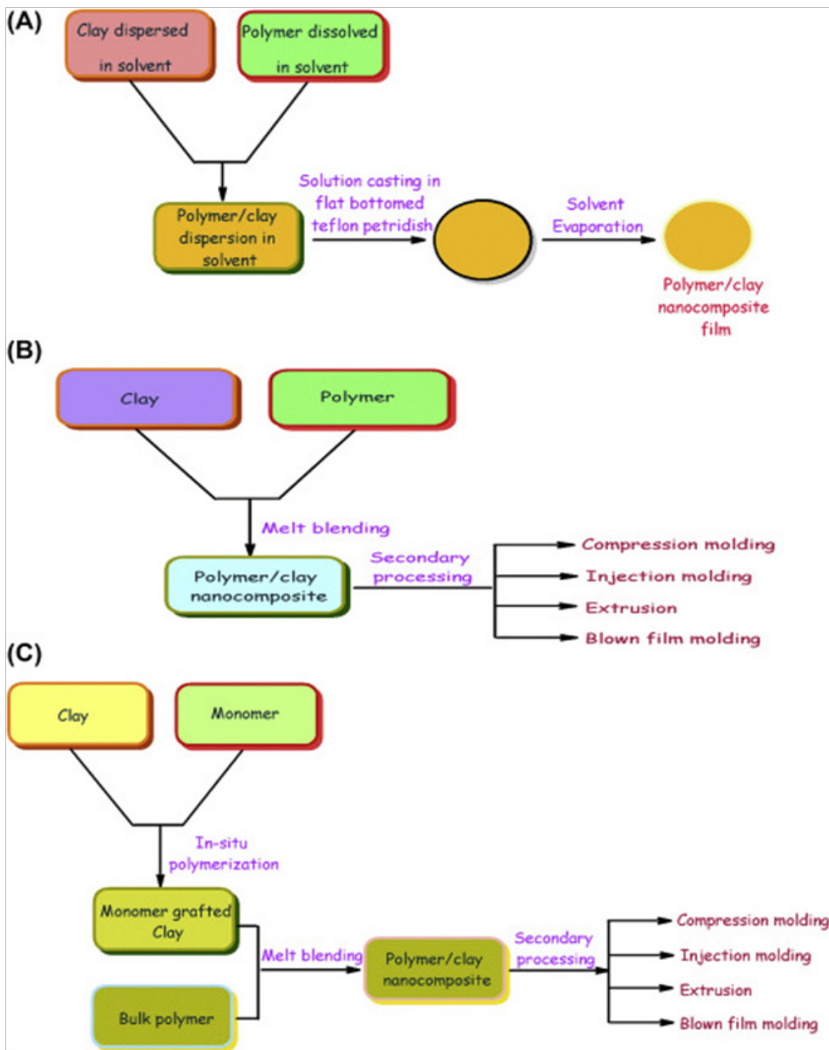
Figure6 Different techniques for the preparation of polymer-clay nanocomposites: (A) solution casting; (B) melt blending; (C) in-situ polymerization.
